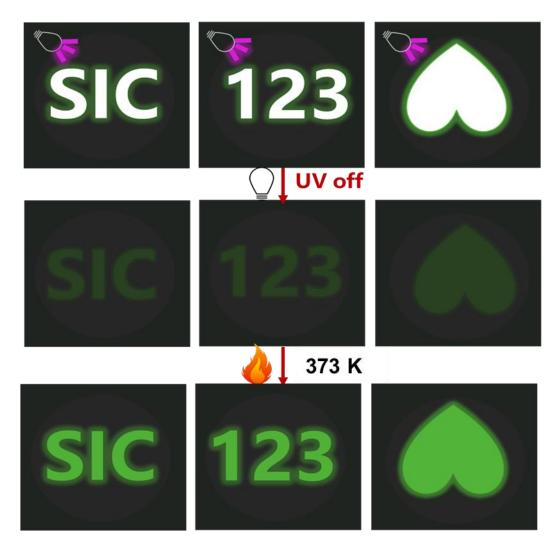
Fig. S21 The process and photos of encrypting and decrypting letters, numbers, and patterns using the  $LiTaO_3$ :1.0%Tb<sup>3+</sup> phosphor.
